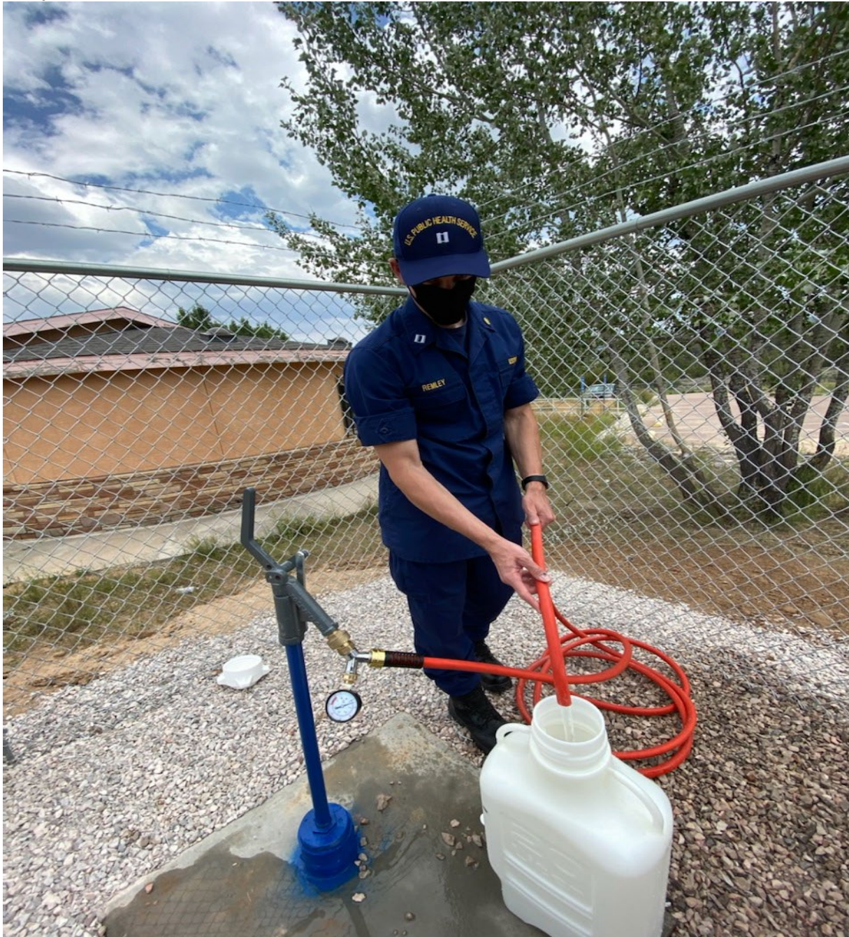
LT Kevin Remley flow testing a transitional watering point as part of the Navajo Water Access Mission.
