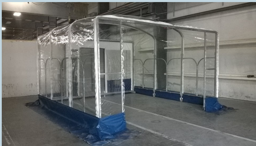
A mobile dust control booth modified and deployed to a stone countertop fabrication shop for field evaluation of its performance in reducing workers' exposure.
