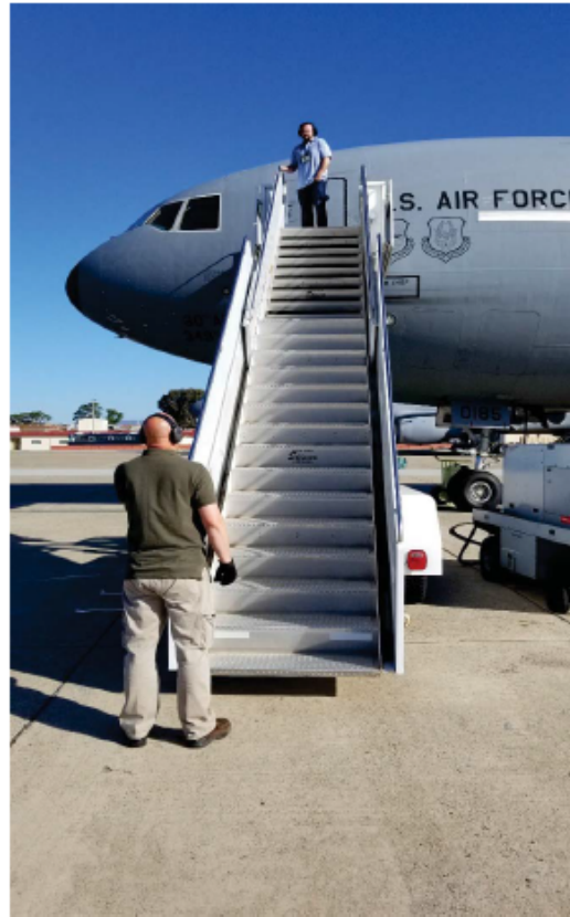
Wide Body Stairs at KC-10, 24 Steps
