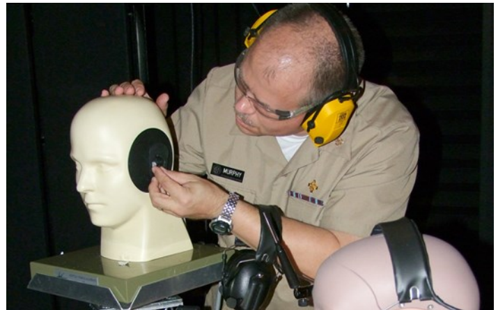
Scientist Officer CDR William Murphy conducting tests on hearing protection devices at the US Army Aberdeen Proving Ground EAR laboratory. (US Army Photo by Ron Carty)
