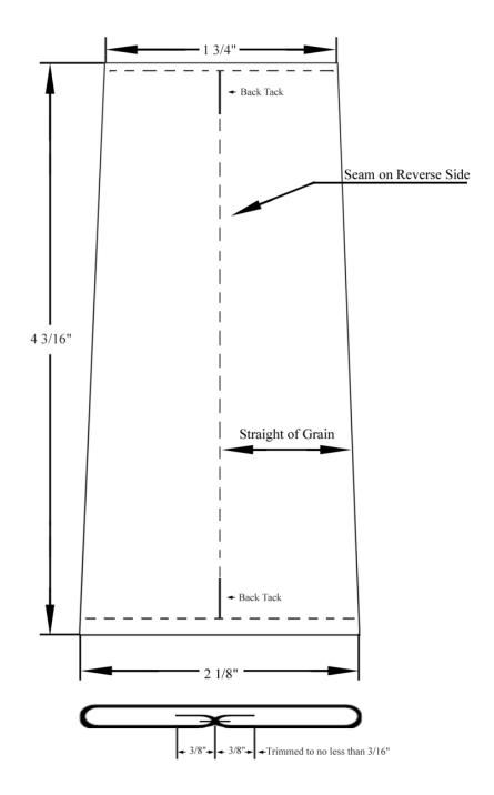
Figure 1 - <u>Soft Shoulder Boards Assembly Details</u>
